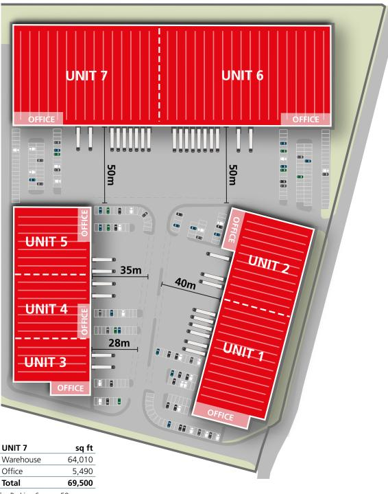
Car Parking Spaces: 58 Dock Levellers: 7 Loading Doors: 2 Eaves height: 12.5m
